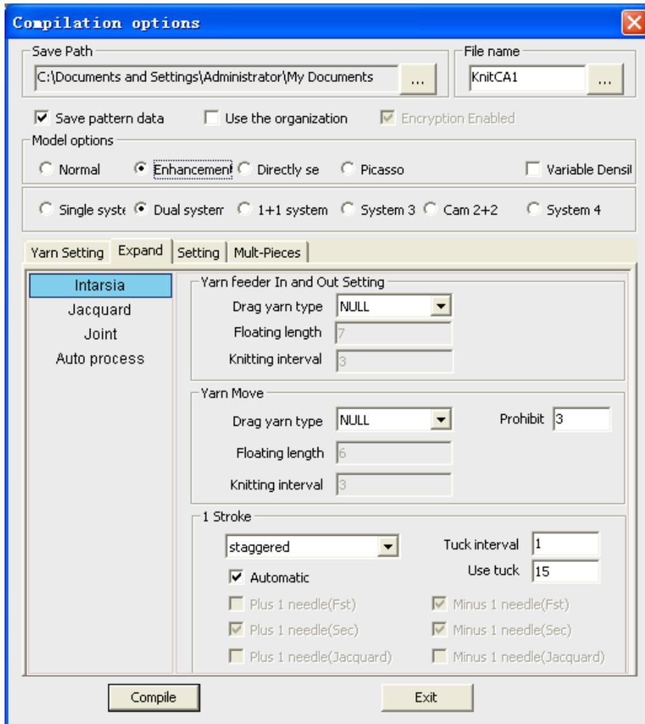
Figure 2 Pattern Expansion Parameter Selection Windows
