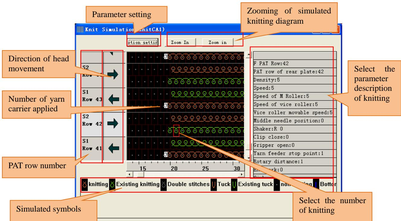
Fig. 6 “Knitting Simulation” Window
