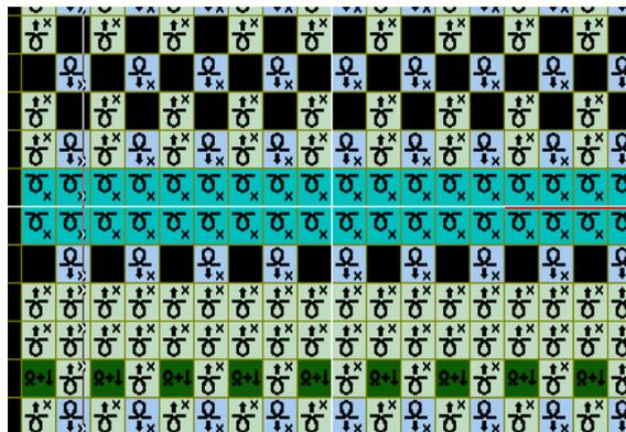
Front cast-off and back comb idle revolution
