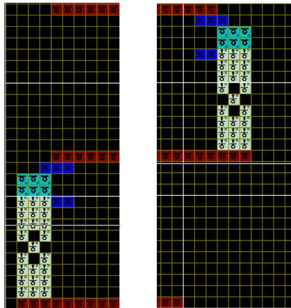
Main yarn doffing (Body yarn carrier knitting and cast-off)
